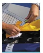
Ensure that the gas cylinder is correctly tightened
