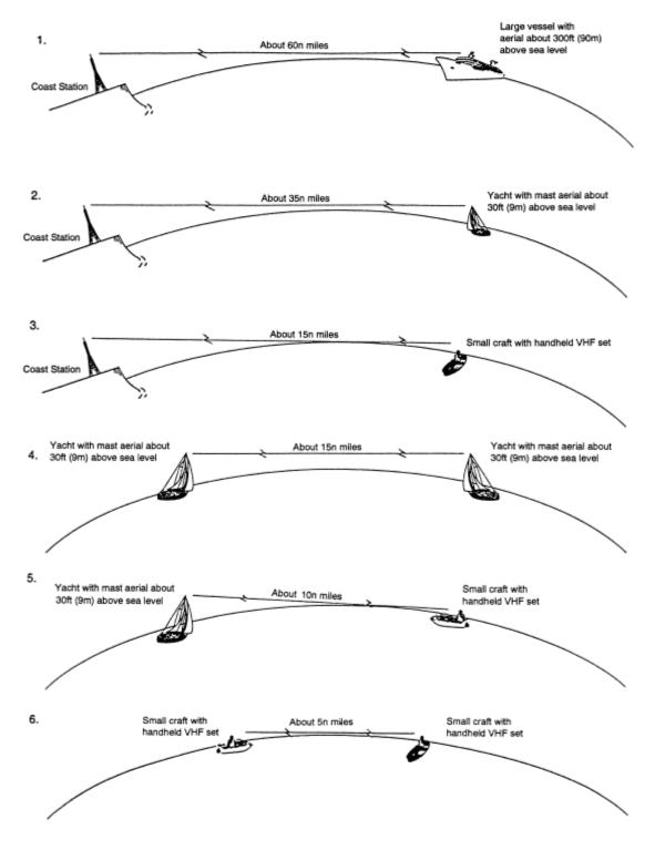
It should be noted that the fact that a transmitter and receiver are within radio sight does not automatically guarantee that an acceptable signal will be received at that point. This will depend, amongst other things on the power of transmission, the sensitivity of the receiver and the quality and position of the transmitting and receiving aerials. The range may also be affected to some degree by the pressure, temperature and humidity of the air between the transmitter and receiver.
