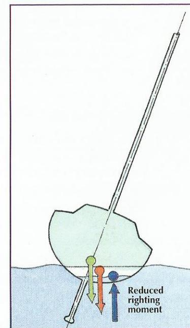
water (see note 5 above). Secondly water trapped high in the vessel raises the centre-of-gravity (see note 1), and its weight also reduces freeboard so that more water is likely to be shipped.
