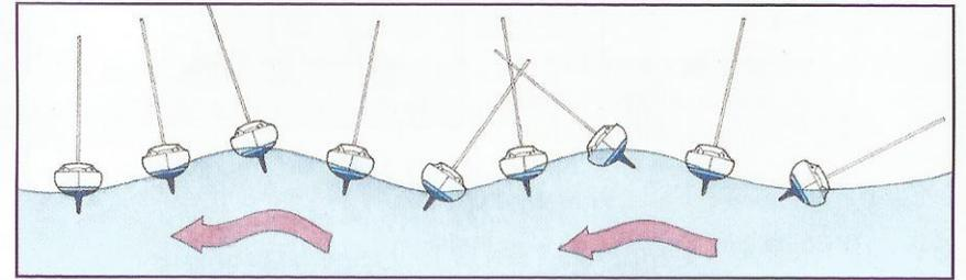
Vessels may experience resonant rolling if encountering a series of fairly regular beam waves. The waves do not have to be especially large, but may just have a period similar to the natural rolling period of the boat. Due to the damping effect of wind in the sails, this is generally of less concern to vessels under full sail.
